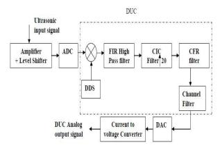
Figure 1. Digital Up Converter Block Diagram
