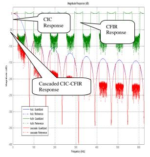
Figure 8.Working of the CIC-CFIR Filter and its Combined Response in MATLAB
